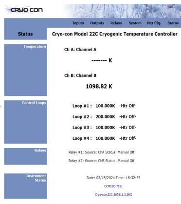
**Utility Software:** Utility software is provided that connects any Windows based personal computer to the Model 22C via any of its remote interfaces. This software provides a graphical control panel that greatly simplifies instrument setup and configuration. Features include:
